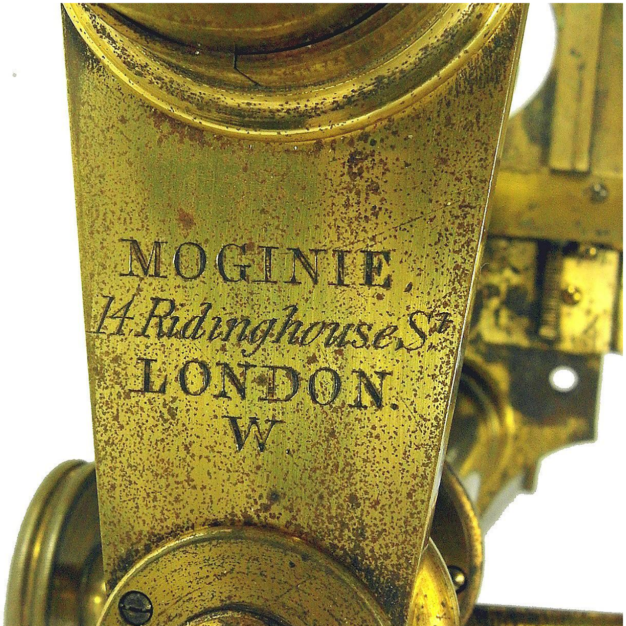
Figure 16. Signature on Moginie bar limb microscope identifies it as being manufactured in 1860s
